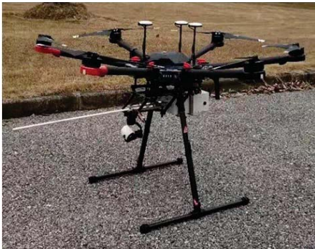
(UAV with exhaust gas testing device)
